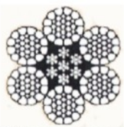
IWRC 6xP·WS(31) Construction 7x7+6xP·WS(1+6+(6+6)+12)
